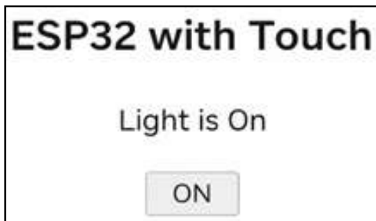
Figure3: ESP32 Touch-Based Web Interface for Light Control
