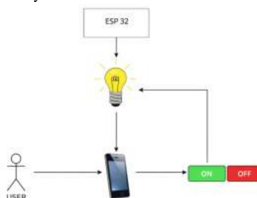
Figure2: ESP32-Based Smart Light Control System Using Mobile Interface
